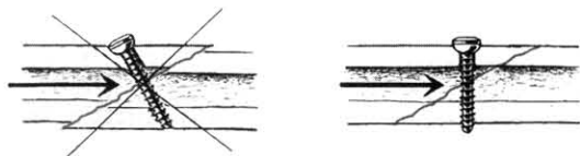
FIGURE 52-10. A lag screw inserted at right angles to the fracture plane provides maximum interfragmental compression but minimal axial stability. Under axial load, one fragment tends to glide on the other with loss of reduction and fixation. If a screw is inserted at right angles to the long axis of the bone, it provides maximum axial stability but tends to cause some dislocation of the fragments as it is tightened. Therefore, it is best to have one screw at right angles to the axis and the others at right angles to the fracture plane (see Fig. 52-11). Reprinted from Müller M, Allgöwer M, Schneider R, Willenegger H: Manual of Internal Fixation: Techniques , p 191, 1979, with permission from Springer-Verlag.
